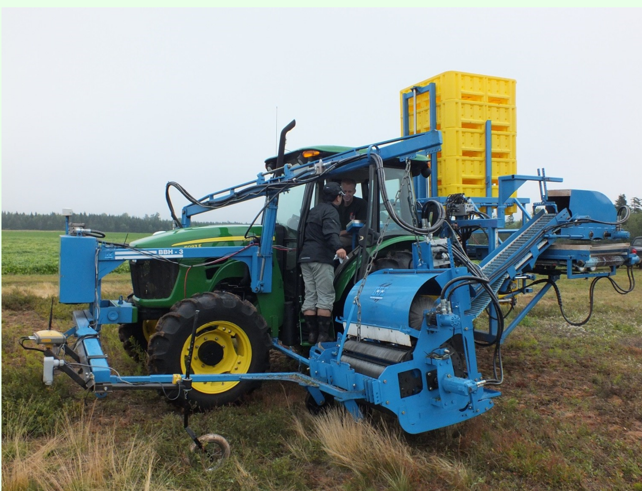
Yield monitoring system, ultrasonic sensor and RTK-GPS incorporated into a harvester
