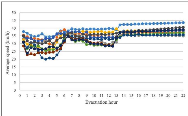
**Figure 7.** Temporal variation of traffic congestion propagation measured in relation to average speed along transit lines.
