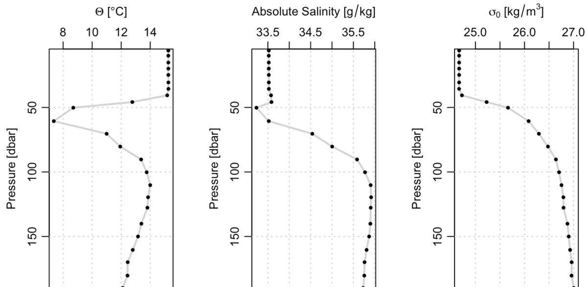
*A near-surface portion of a profile sampled in November of 2015, with a drifting Argo profiling float that was in water approximately 2 km deep, above the abyssal plain to the south of Halifax. The patterns hold several clues about the dynamics underlying the space-time variability of the ocean system.*
