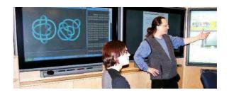
One central feature of the laboratory is the large (60 and 72 inches diagonal) tiled multi-touch sensitive, high-resolution display panels that permit users and researchers to interact directly with the panels rather than through the usual keyboard or mouse. In addition, there are a variety of stereo visualization devices and multicast AccessGrid capacity for computing and grid collaboration. A proportion of the budget is earmarked for a refresh of equipment in this
