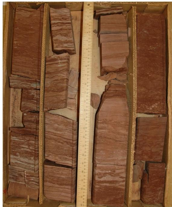
Figure 1.8: Core collected from the Eurydice P-36 well. A total of eight boxes of core are shown and labeled. A meter scale is placed between the two boxes in each image for scale. The core can be viewed at the CNSOPB's GRC in Dartmouth, NS. The top of the core is at the top-left and base at the bottom-right. **Geologic Overview**
