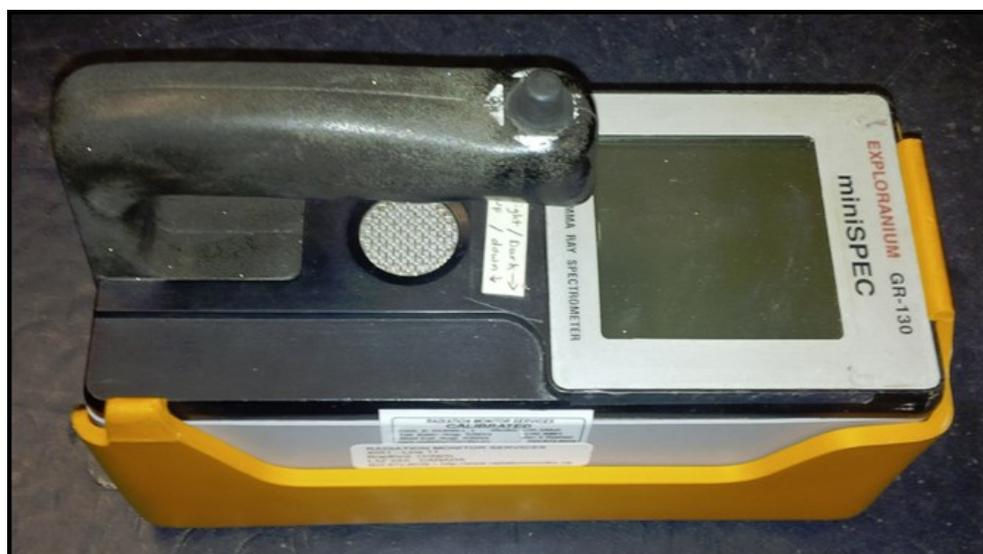
*Figure 3.9: Photograph of the Exploranium GR-130 miniSPEC scintillometer. The device is a single unit with a LCD screen, a handle with a controlling nub, and a signal-to-noise apparatus (silver circle beneath the handle).*
