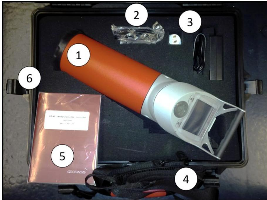
*Figure 3.10: Photograph of the GEORADiS GT-40 Multipurpose Gamma Center and associated parts (1. The scintillometer, 2. The usb connective cord, 3. The power adaptor, 4. The carrying strap, 5. The user's guide, and 6. The protective carrying case)*
