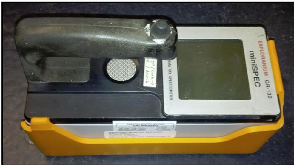
*Figure 3.9: Photograph of the Exploranium GR-130 miniSPEC scintillometer. The device is a single unit with a LCD screen, a handle with a controlling nub, and a signal-to-noise apparatus (silver circle beneath the handle).*
