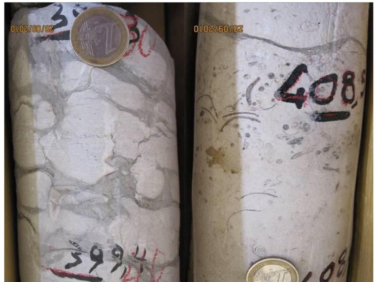
Figure 45: Gândara formation limestones in MRW-8 well cores.
