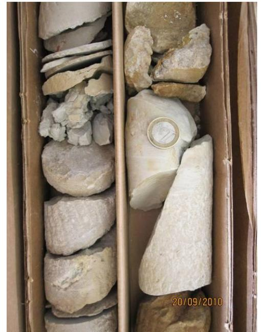
Figure 44: Cacém formation limestones in MRW-2G well cores.
