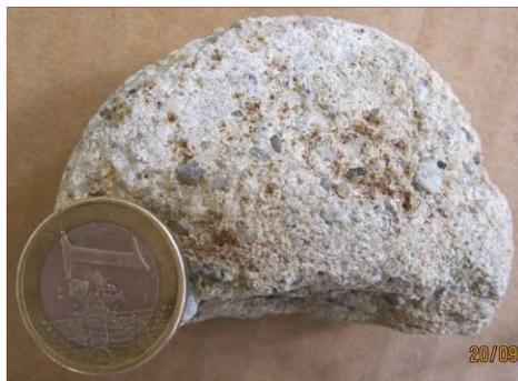
Figure 42: Torres Vedras sandstone in MRW-9 well cores.
