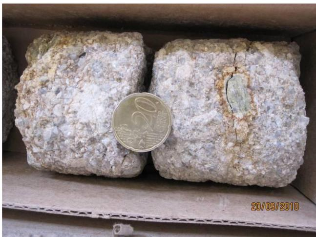
Figure 35: Abadia formation coarse arkosic sandstones in Ar-1 well cores.
