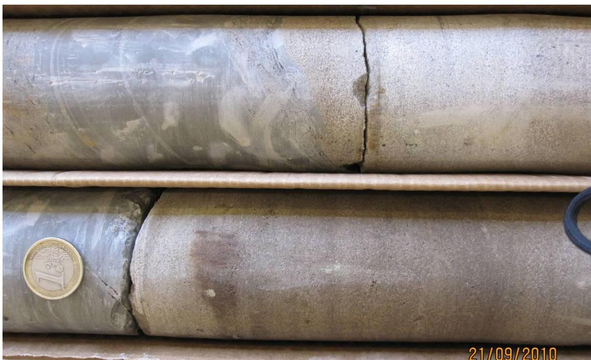
Figure 56: Abadia fm oil impregnated sandstones in FR-3 well cores.
