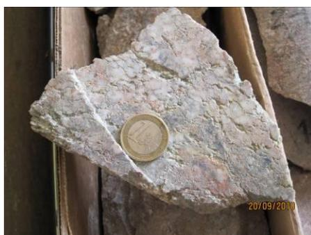
Figure 5 & 6: 17C-1 well granite cores.
