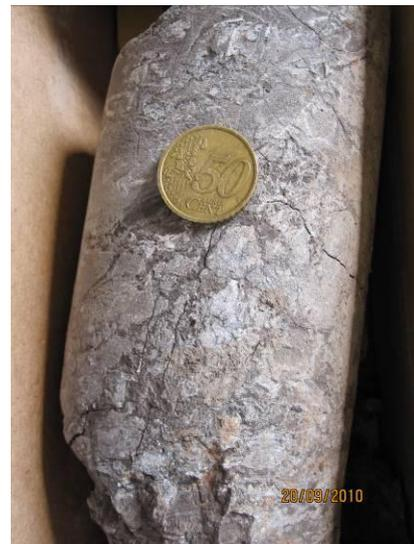
Figs. 20 & 21: Brenha formation shaly limestones in MRW-9 well cores.
