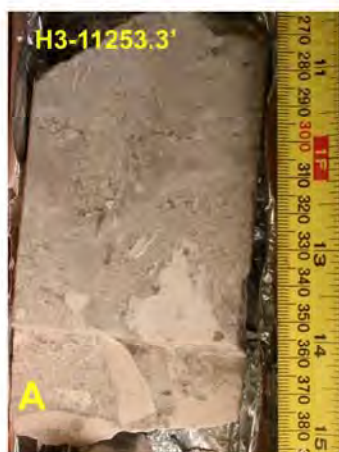
A- angular bioeroded stromatoporoid (cream) & microbial? clasts in skeletal-fragmental grainstone-packstone
