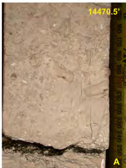
Lithoclast floatstone of early cemented broken microbial crusts, some clast edges bioeroded possibly when hardground. White tiny fossils typically Tubiphytes .
