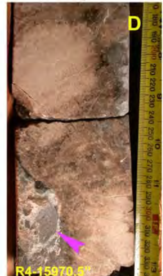
D- Recrystallized (?leached??) large head coral. Note late dolomite in fractured/brecciated matrix with calcite cement lining
