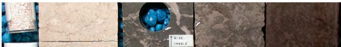
Figure 6 Southwest to northeast colour comparison of Abenaki lithofacies A) ooid grainstones and B) microbolites (thrombolites). Albatross B-13 core 1 (in A) and cuttings (in B) and Acadia K-62 core 5 of Western Shelf, Demascota G-32 core 5, Panuke F-09 and M-79 sidewall cores, Penobscot L-30 cores (1 in A, 2 in B), and West Venture C-62 core 13 of Panuke Trend to Sable Delta.
