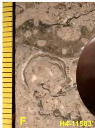
F- bored hexacoral? clast (dark) above attached to multi-layered mollusk? with cellular wall structure suggestive of rudistid bivalve (white and dark semicircular fossil ~ 10 mm across) in skeletal-oolitic grainstone
