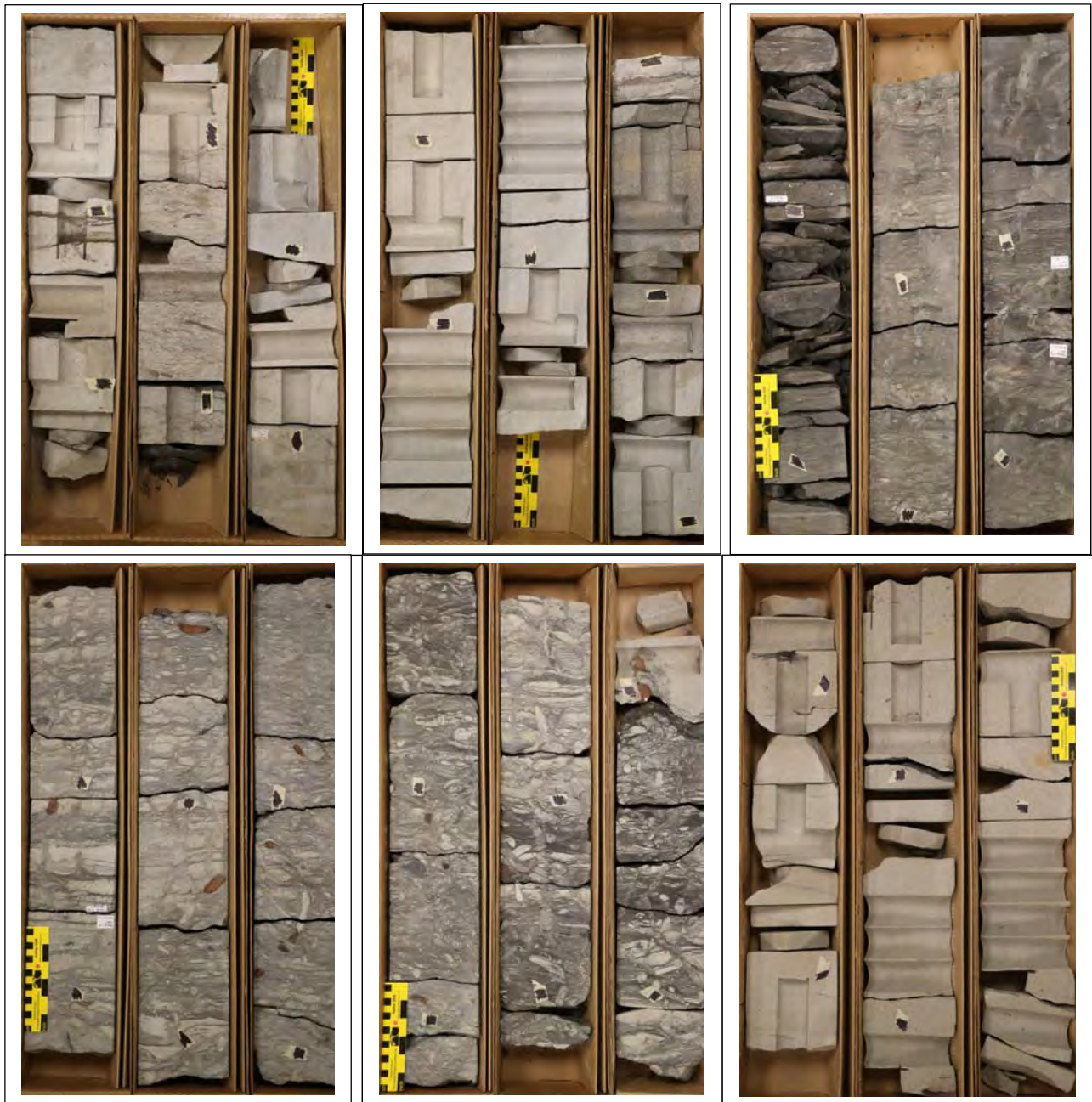
Figure 4: Photo compilation of slabbed core from the Thebaud I-93 well's core No. 1 (3065.68-3081.27 m MDRT). The small white squares with black markings indicates the point where X-ray fluorescence XRF measurements were collected for rock classifications according to Herron (1988). Though comprising only a short interval with minimal recognizable change in depositional environments, analyzing the physical rock characteristics and grain size distribution provided further information with regards to the energy level at different depths and how this transitioned upwards through time. Scale bar is 15 cm / 6 inches long.
