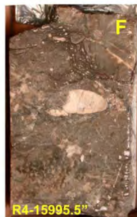
G- recrystallized large gastropod-bivalve fragments among reef debris and oncoids(?)
