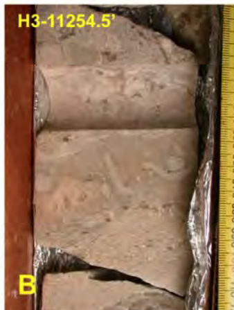
B- recrystallized (leached?) hexacoral clast with sediment filled borings in micritized skeletal-fragmental superficial ooid grainstone
