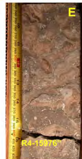
E- branching and massive coralline sponges (stromatoporoids) in reef framestone
