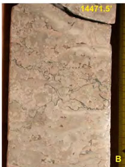
Thrombolitic textures with plentiful shelter cavities and geopetal fill (stromatactid fabric), tubular forams -serpulids (nubeculinellids?) part of micritic linings of cavities
