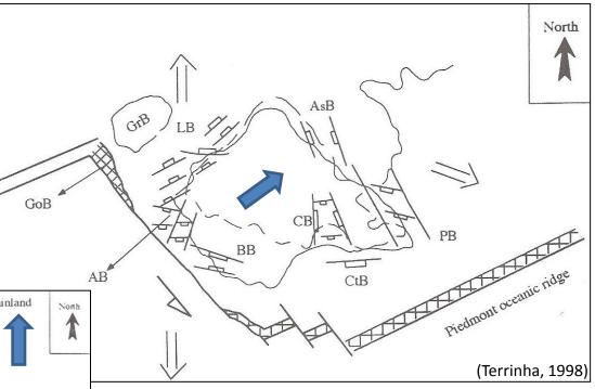
During Mesozoic extension, N-S to NW-SE faults acted as right lateral transfer faults, separating elongated tectonic blocks. These two directions, NE-SW dip-slip faults and NNW-SSE transfer faults, may also be recognised in the palaeogeographic evolution of the Algarve Basin during the Jurassic and Cretaceous.
