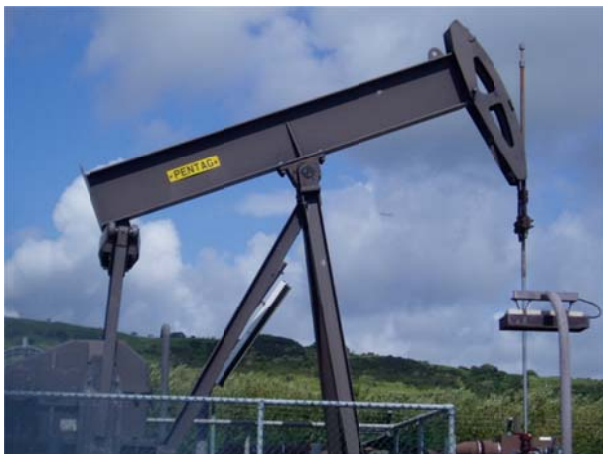
Figure 2: The well in Kimmeridge Bay. This is a beam pump, also called a nodding donkey.
