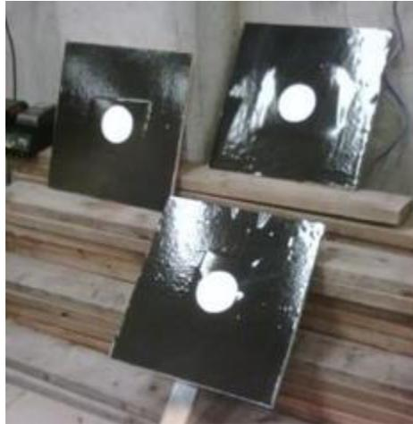
Figure 2.4 – Targets used for georeferencing. The targets have high reflective background (reflective black) contrasted with a less reflective centre circle, design by Johnathan Thibodeau.
