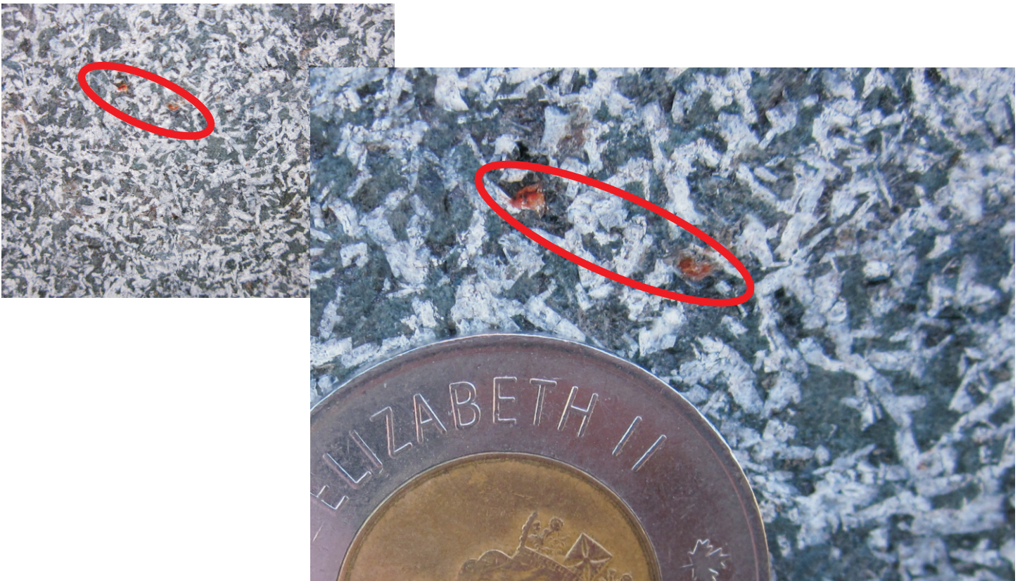
Rusty Altered Olivine Grains in the Ritcey Headstone
