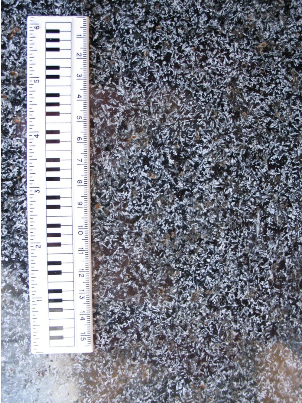
The distinctive "snowflake" texture of the Titanic headstones, caused by random orientations of plagioclase crystals.
