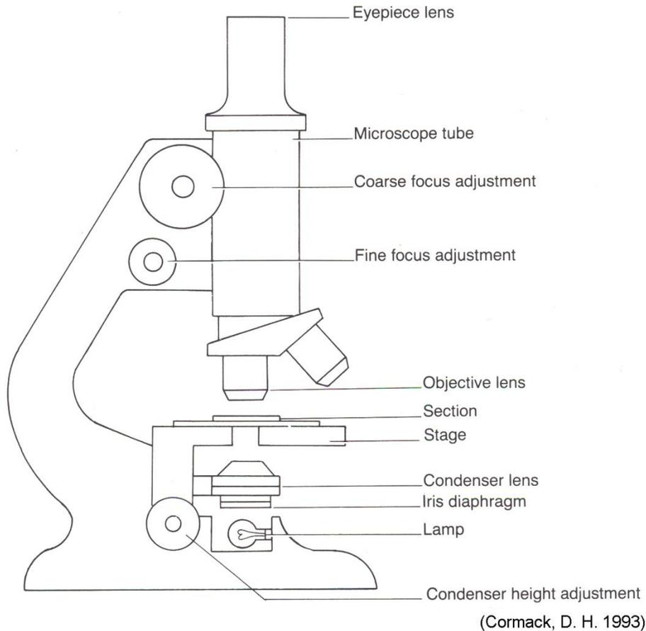
Parts and simplified optical path of the light microscope.
