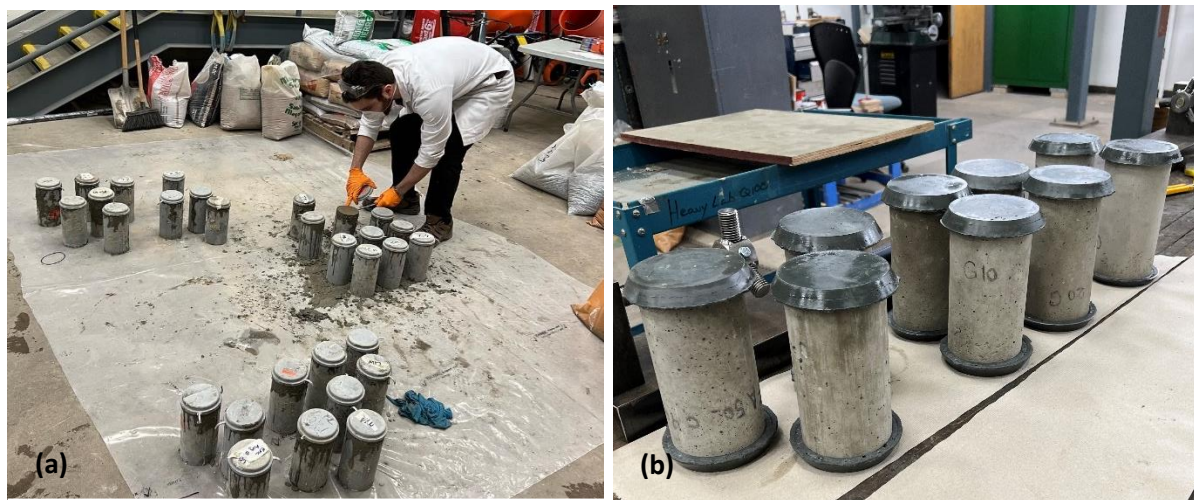
Figure 6: a) Casting concrete in molds and preparing specimens. b) Capped specimens
