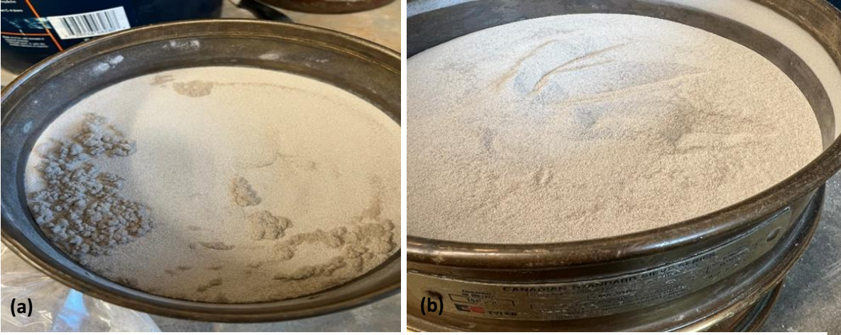
Figure 5: Retaining gypsum powder on sieve No.100 after shaking. a) wet gypsum, b) dry gypsum
