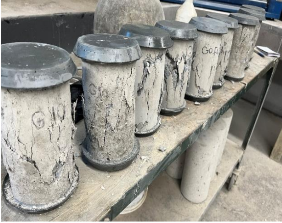
Figure 7: Specimens after compressive strength test
