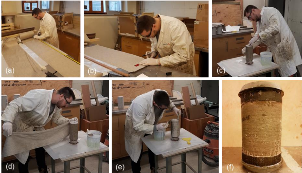
Figure 1 – Specimen Preparation: (a) Cut Flax Fabric to Length; (b) Measure and Cut Flax Fabric to Correct Width; (c) Apply Coat of Epoxy to Concrete Cylinder; (d) Apply Flax Fabric to Wetted Cylinder; (e) Apply Epoxy to Surface of Flax Fabric; (f) Finished Wrapped Specimen
