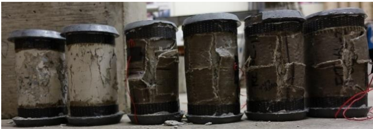
Figure 4 – Tested Specimens (from left to right: FCC-0L-1, FCC-0L-2, FCC-3L-1, FCC-3L-2, FCC-6L-1, FCC-6L-2)
