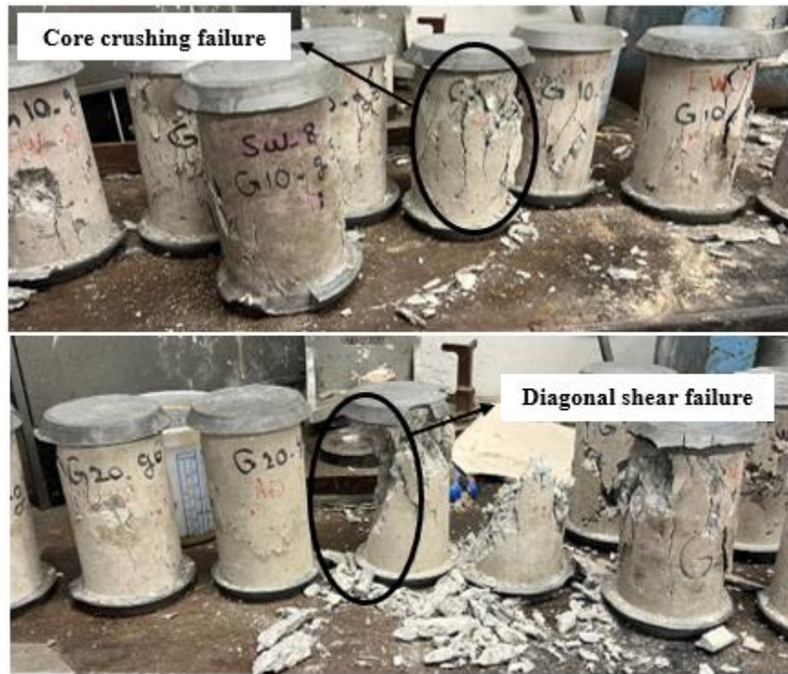
Figure 4. Typical failure modes of the specimens after compressive strength test.
