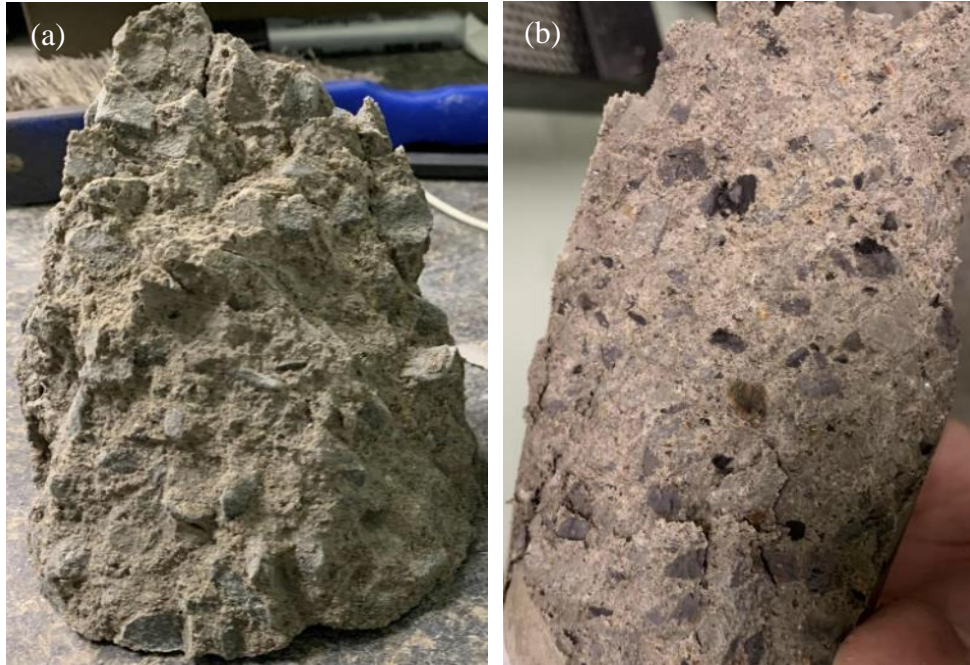
Figure 1. fracture plane of the unconfined concrete specimens from load-controlled axial compression testing: a) normal density concrete cylinders and; b) lightweight aggregate concrete cylinders.
