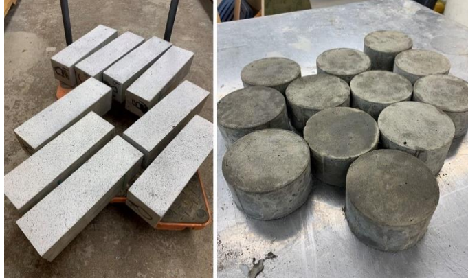
Fig. 1. Specimen fabricated for testing, a) prism specimens and, b) disk shape specimens
