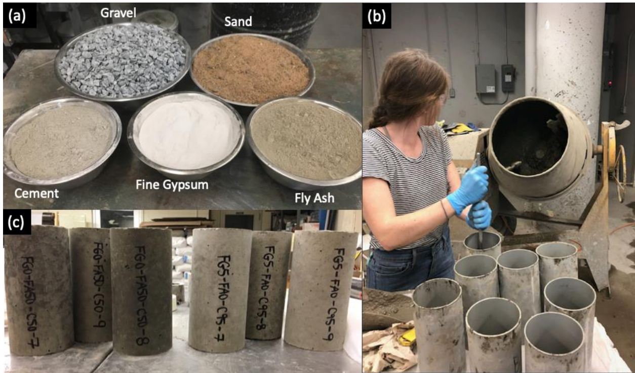
Figure 3. Specimen preparation: (a) dry materials; (b) hand tamping; (c) comparison of specimens with and without fly ash
