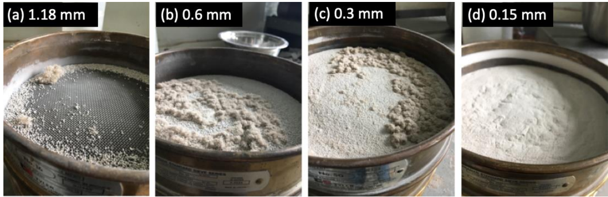
Figure 1. Gypsum retained on sieves (a) No. 16; (b) No. 30; (c) No. 50; (d) No. 100
