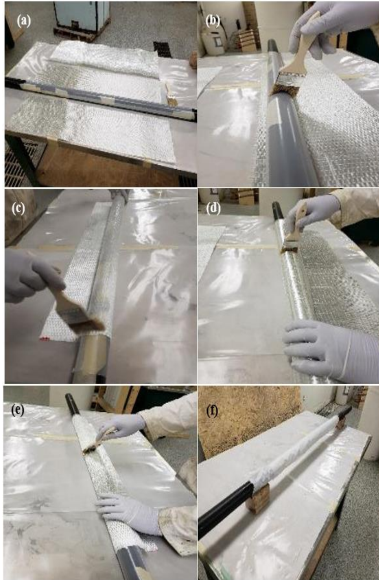
Figure 2 Fabrication of GFRP pile specimen: (a) material used for fabrication; (b) brushing the surface of the plastic pipe gently with epoxy resin and hardener; (c) brushing the first (90-degree hoop) layer of glass fabric with resin; (d) adding resin to the second and third (0-degree axial) layers of glass fabric; (e) adding resin to the last (90-degree hoop) layer of glass fabric; and (f) wax paper wrapped around the GFRP pile after completion of the pile layers
