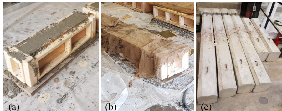
Figure 3. Concrete columns: (a) fresh concrete, (b) curing, and (c) concrete specimens - Courtesy of Koosha Khorramian.
