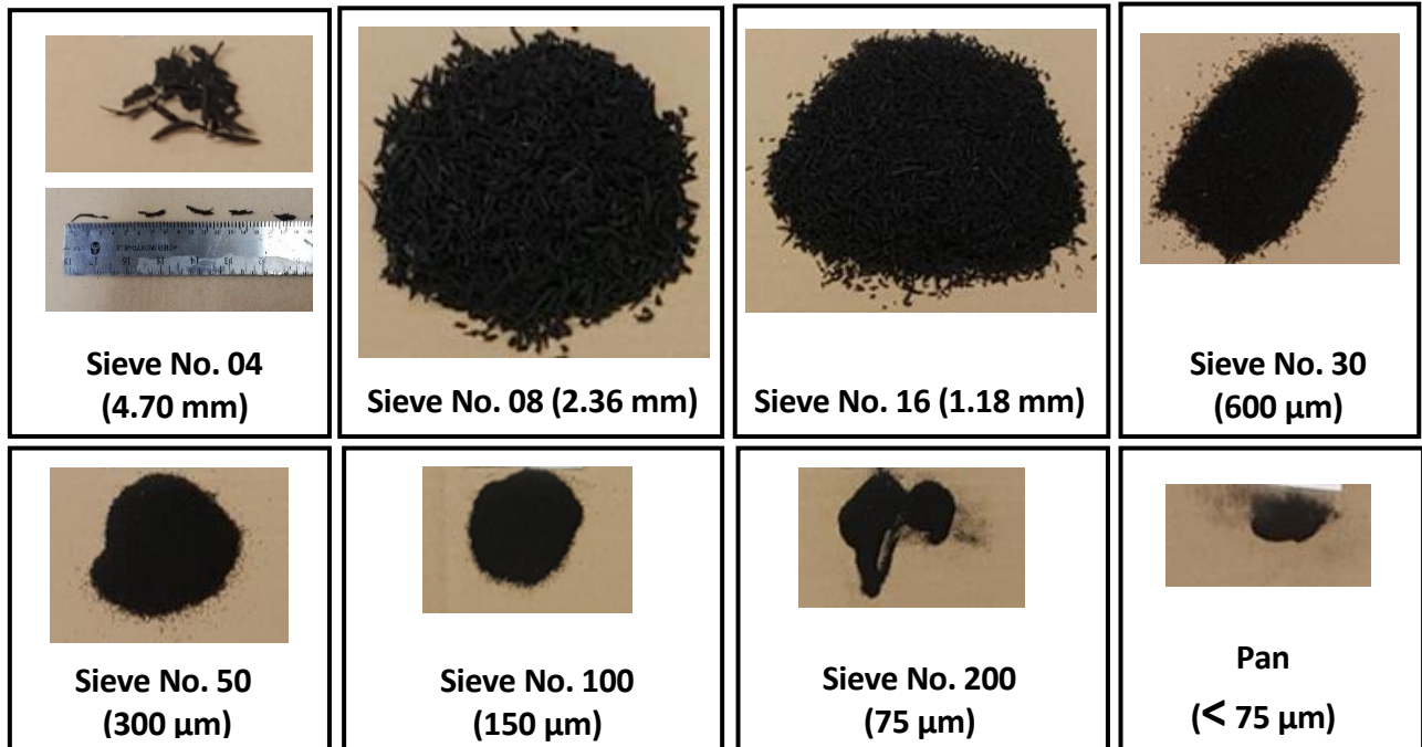
Figure 1: Various sizes shredded rubber particles remained on sieve#4, #8, #16, #30, #50, #100, #200, and Pan
