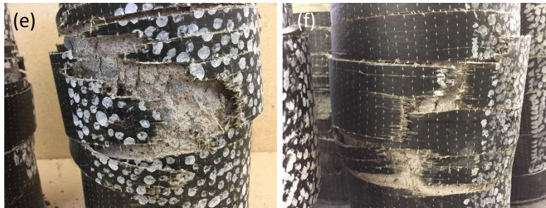
648 Figure 4. Test specimens after failure: (a) plain group; (b) L2 group; (c) L4 group; (d) L6 649 group; (e) and (f) typical rupture of hoop fibers. 650
