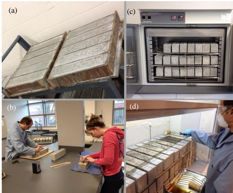
Figure 2. Specimen preparation: (a) formwork; (b) surface preparation; (c); oven drying; and (d) applying FRP.
