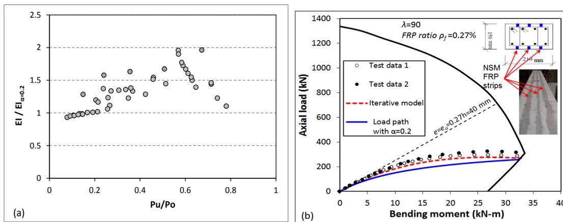
Fig. 3 – (a) Variation of  $EI / EI_{\alpha=0.2}$  versus load capacity ratio; (b) comparison of load path with  $\alpha=0.2$  with experiment (Gajdosova and Bilcik 2013) and iterative model (Sadeghian and Fam 2014).
