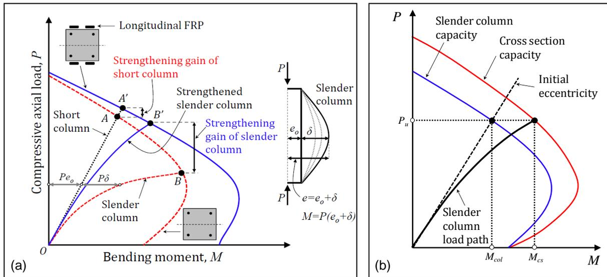
**Fig. 1 – (a) Performance of short and slender RC columns before and after strengthening with longitudinal FRPs; (b) relationship between cross section capacity and slender column capacity.**
