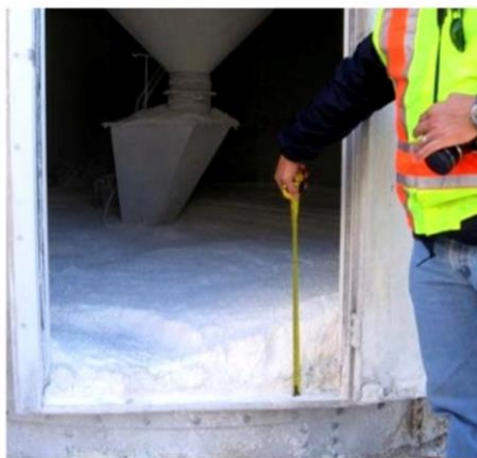
Cornstarch accumulation under cornstarch silo
