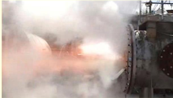
Corn Flour Explosion with Relief Venting
