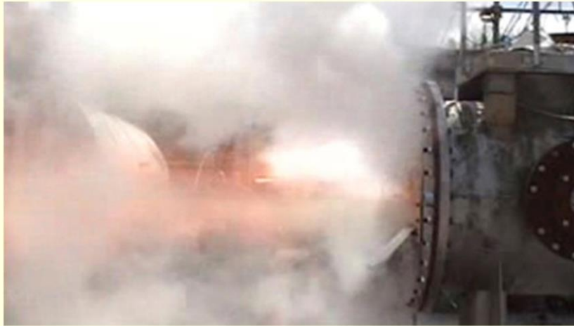
Corn Flour Explosion with Relief Venting
