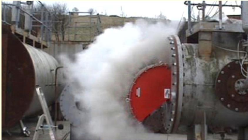
Corn Flour Explosion with Flameless Venting
