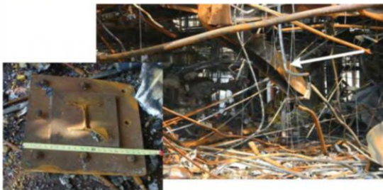
Support Column Sheared Off Baseplate
