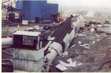
Methane-triggered coal dust explosion - Westray Coal Mine (26 fatalities)
