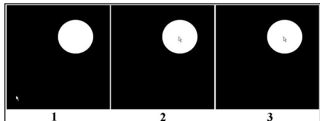
**Figure 4: Snap-to-target: (1) Cursor begins to approach target; (2) Cursor reaches 90% threshold and immediately snaps to centre of target; (3) Cursor remains snapped to target centre until pointer moves outside of 90% range**
