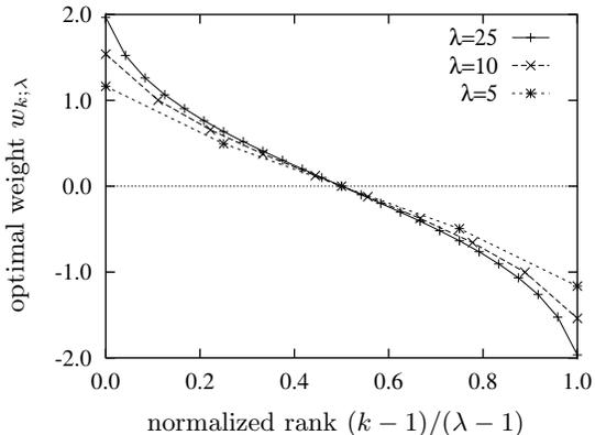
**Fig. 2.** Optimal weights  $w_{k;\lambda} = E_{k;\lambda}$  plotted against the rank  $k$  of a candidate solution in the set of offspring for several values of  $\lambda$ . The ranks have been scaled linearly to fall in the range from zero to one. Note that only the points, not the connecting lines, are of practical significance.
