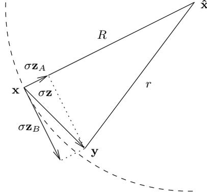
**Fig. 1.** Decomposition of a vector  $\mathbf{z}$  into central component  $\mathbf{z}_A$  and lateral component  $\mathbf{z}_B$ . Vector  $\mathbf{z}_A$  is parallel to  $\hat{\mathbf{x}} - \mathbf{x}$ , vector  $\mathbf{z}_B$  is in the hyperplane perpendicular to that. The starting and end points,  $\mathbf{x}$  and  $\mathbf{y} = \mathbf{x} + \sigma\mathbf{z}$ , of vector  $\sigma\mathbf{z}$  are at distances  $R$  and  $r$  from the optimizer  $\hat{\mathbf{x}}$ , respectively.
