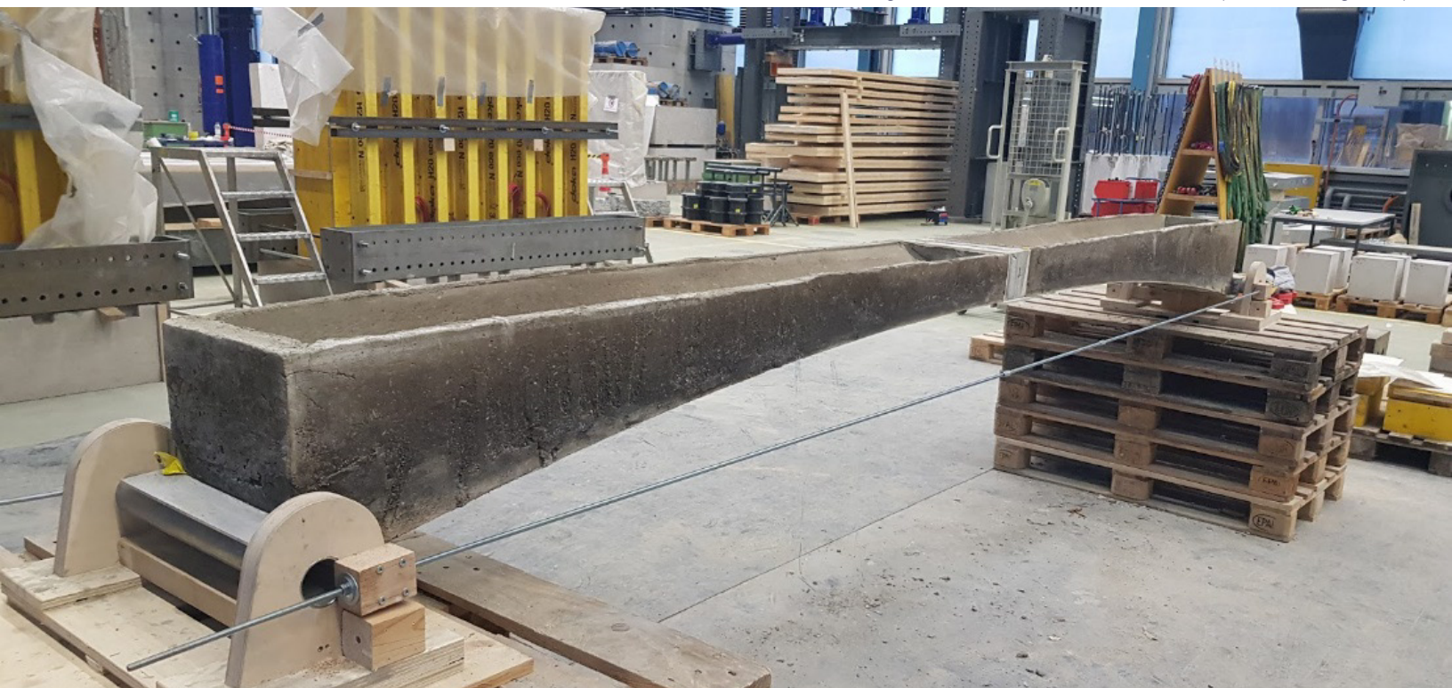
Four meter span prototype. Block Research Group, Image from "When low strength materials meet funicular structures" (IOP Publishing, 2020)
