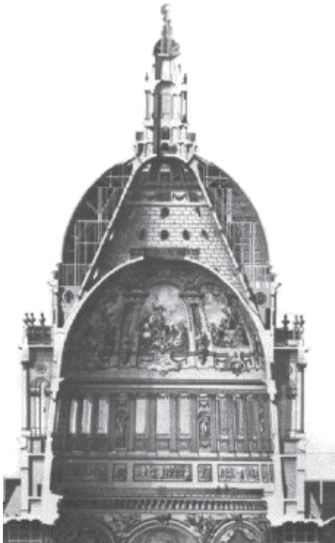
St Paul's Cathedral, London, late 17th century. Cross-section showing the brick cone between the inner and outer domes.
