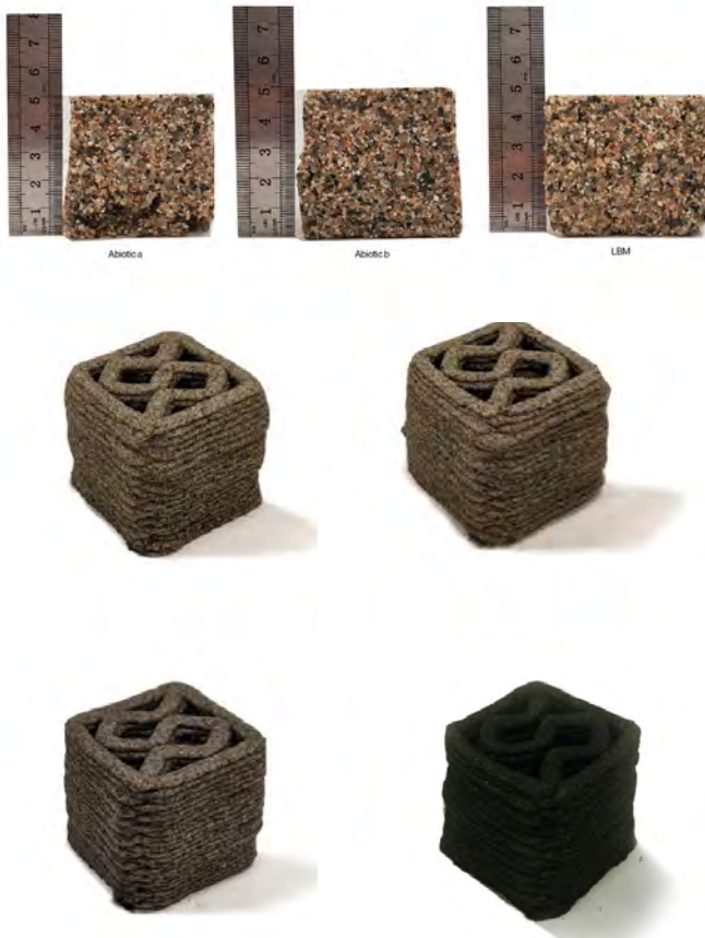
Living Building Material (LBM) specimen (top); Additive manufactured biopolymer binder-aggregate composite specimens. Esther Fu, Gabriel Malo, Rodrigo Guerreiro, image from "Strategies for reducing your project's embodied carbon" (Build Green Atlantic, 2023).
