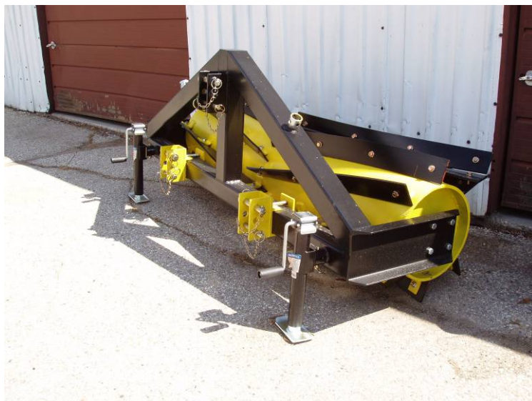
Crop roller: this research-scale blade roller was used to terminate an oat-pea green manure in 2006
