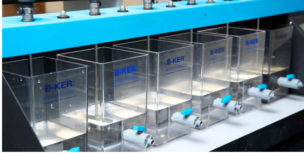
▲ Jar testers used to simulate treatment scenarios before they are sent to pilot-scale
