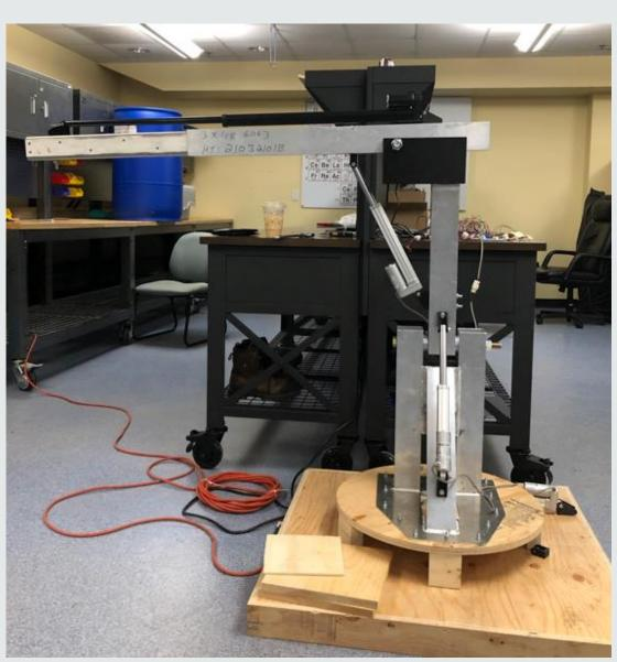
An Arduino controlled scale model was constructed by Team 25 with aluminum used as the primary material. It successfully deploys and collapses in the same manner that the full-sized model will – using four linear actuators to enable the rotation of different sections of the PTL.
