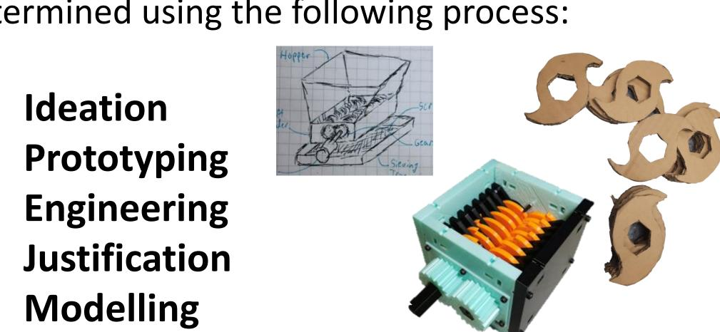
Each subsystem was then tested, improved, and integrated with the other steps.
