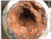
Figure 1: Cross-sectional view of pipe containing biofilm
