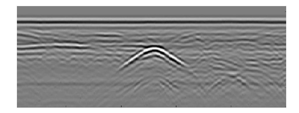
There are many external factors that affect GPR detection and can hamper data gathered at a site: Some factors include decomposition, depth of burial, soil type and disturbance, any other additional items added to the grave, any past or current infrastructure on site, etc.
