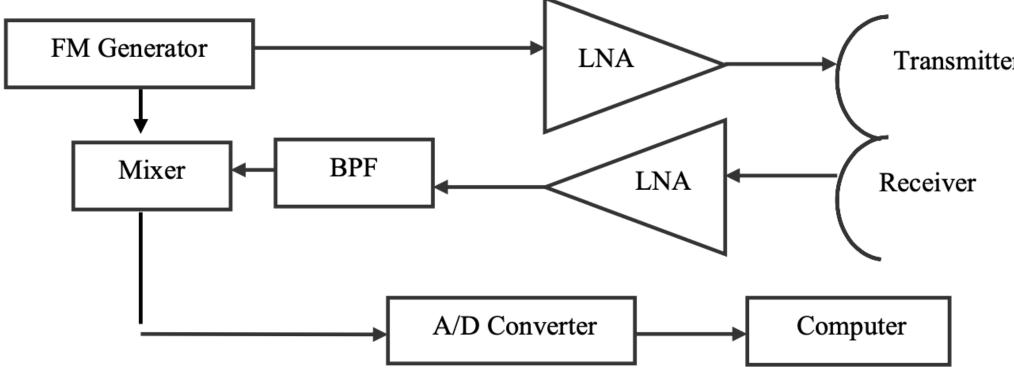
The FM generator outputs a modulated continuous wave signal that is applied to the low noise amplifier (which amplifies it) and the mixer. The transmitted signal is then detected by the receiving antenna and again amplified by another low noise amplifier. The received signal is filtered using a bandpass filter, to narrow the range of frequencies and sent to the mixer. The signals are then sent through an analog to digital converter and manipulated further on the computer.
