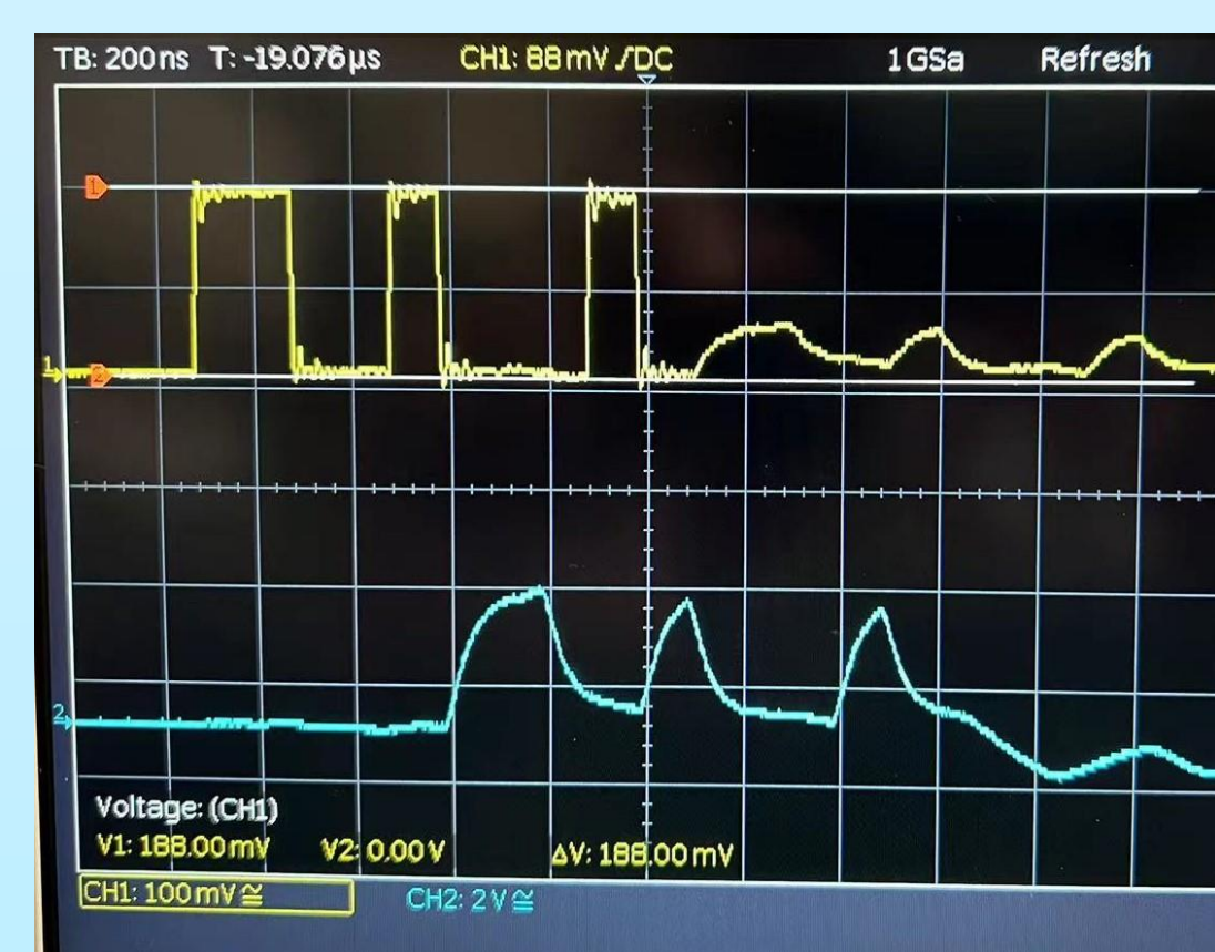
Received Signal Amplitude decreased 40%-50% Delay 520ns Distorted a lot at 10MHz
