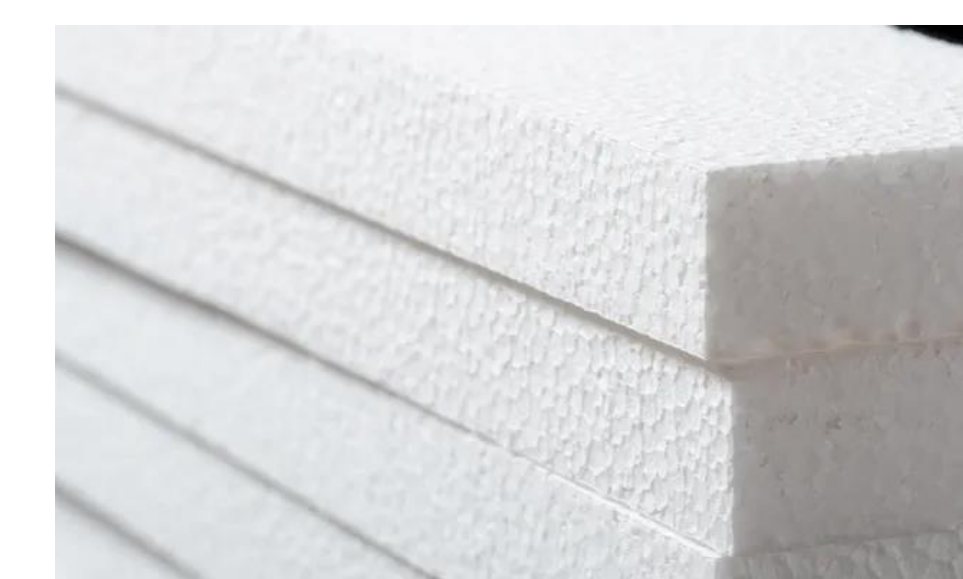
Figure 6. Polystyrene Insulation (Nuclear-Power, 2022)
