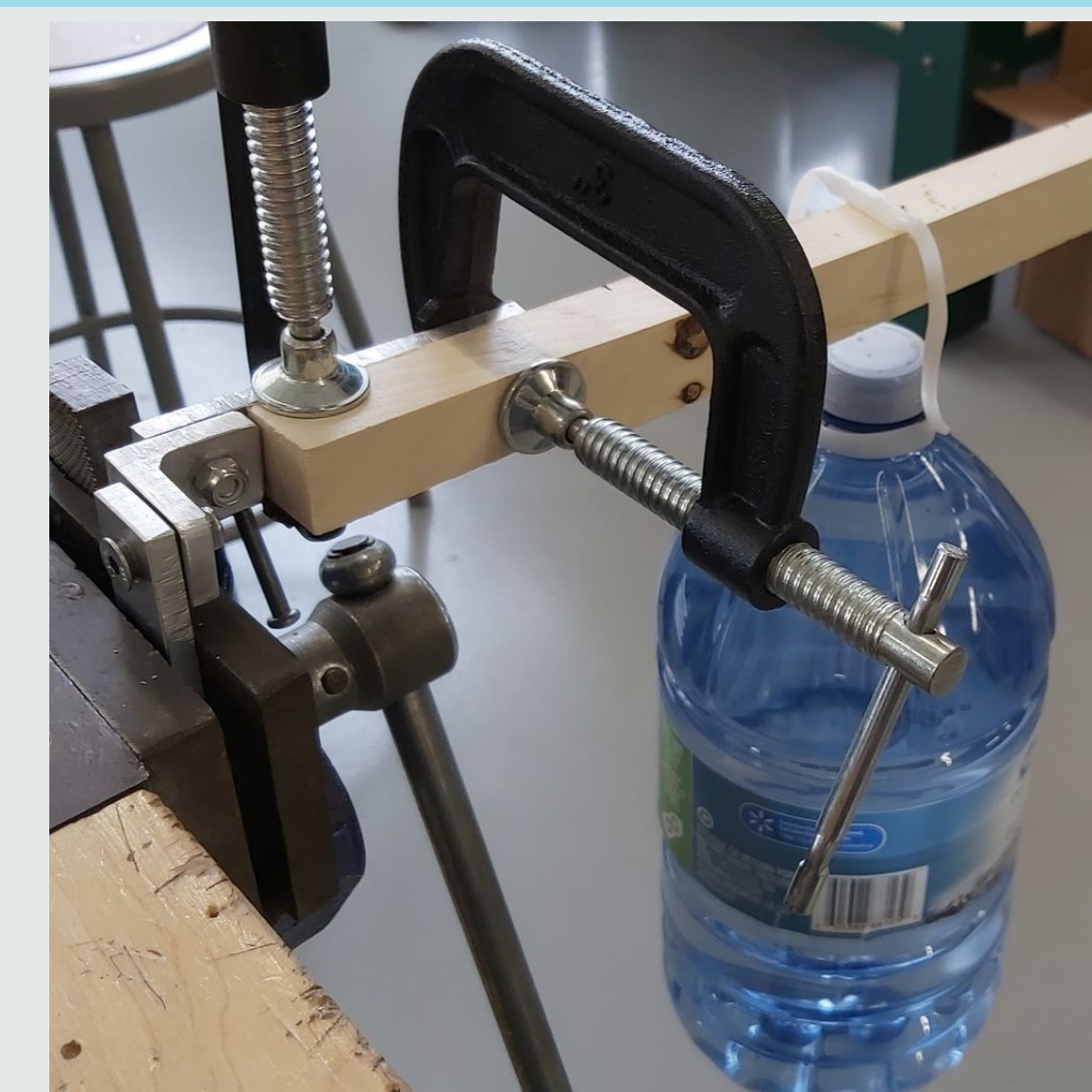
Test apparatus (water bottle used for weight)
