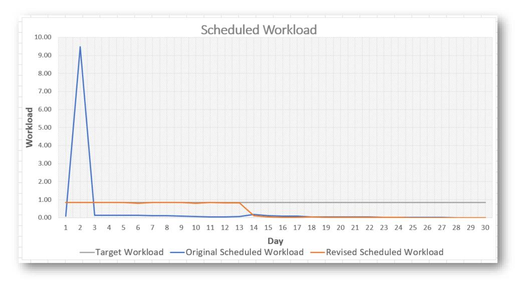
In the above graph, workloads above 1 represent more work assigned on a day than labor available. A user adjustable target of 0.85 is set in the model to avoid queues that could occur when maximally scheduling available labor. Blue line shows the initial assignment's workload as set by the internal database, which exceeds available labor. The orange line shows the model schedule which stays under the target while still ensuring work completed before it's required.
