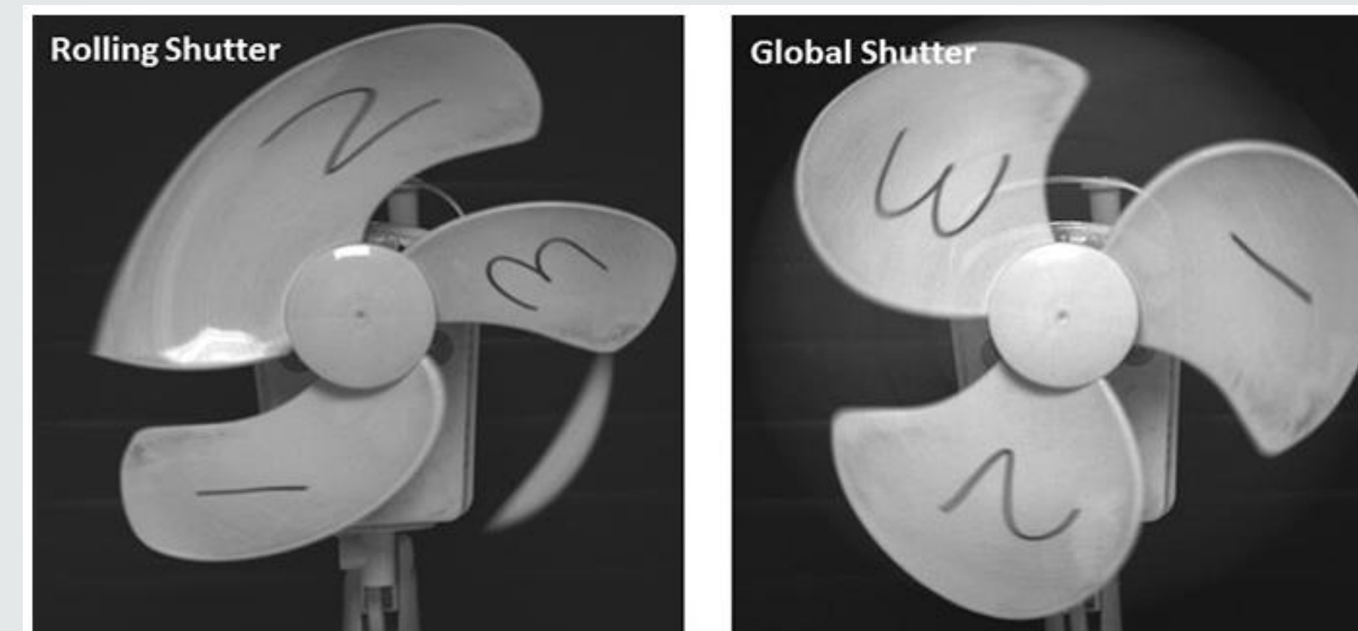
Figure 4: Rolling Shutter vs Global Shutter Image courtesy of andor.oxinst.com
