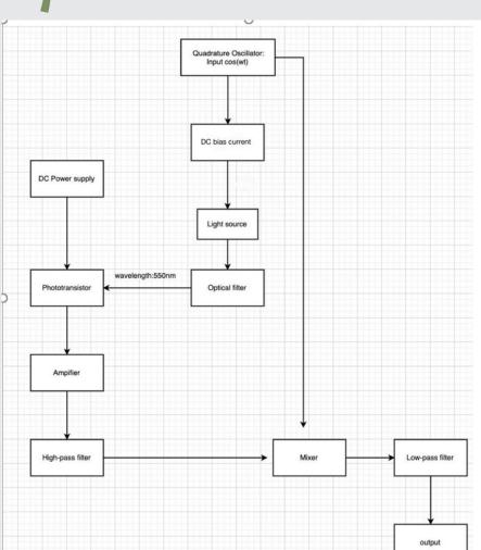
The signal generated by quadrature oscillator go through DC bias current and LED. If the signal doesn't go though DC bias, the led will not be drives. the DC bias current is to increase all voltage higher than zero. Phototransistor receives the light and turn it to digital signal and the amplifier amplify this digital signal .The high pass filter reduce the noises due to sunlight. The digital signal and the original signal generated by oscillator multiply, and the output
