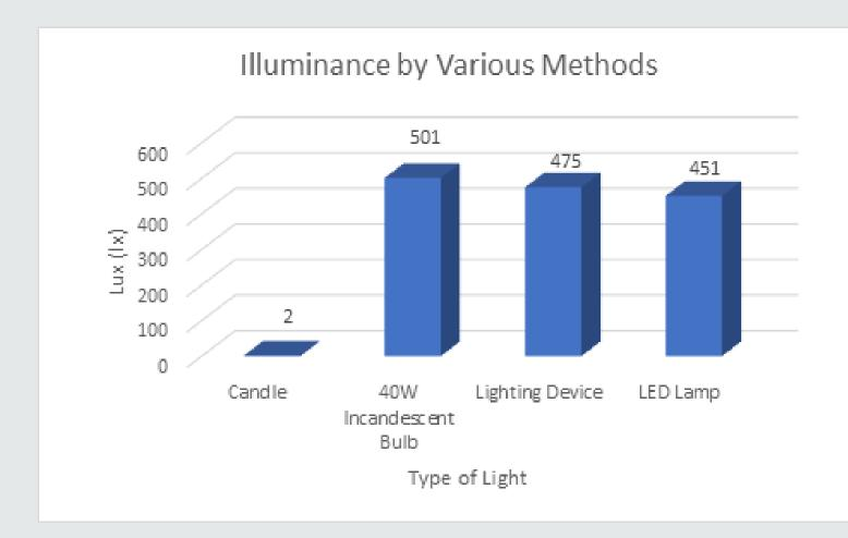
The table on to the left compares our designs luminous flux per unit area (Lux) output to that of similar means of light, as well as the Lux of a candle, which is currently a common source of light in LDCs. This data illustrates that the light produced from our design is in line with that of conventional lighting devices in more prosperous countries. Furthermore, the design vastly outperforms the candle in luminance by over a factor of 230.
