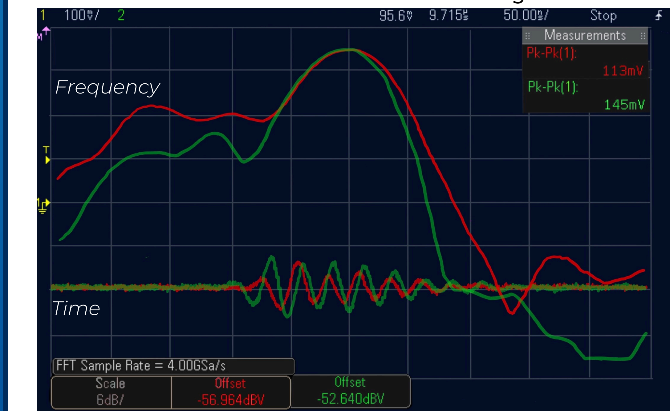
Freq. domain tuned pulse has sharper peak (bandwidth increase) Time domain tuned pulse has higher amplitude (sensitivity increase)
