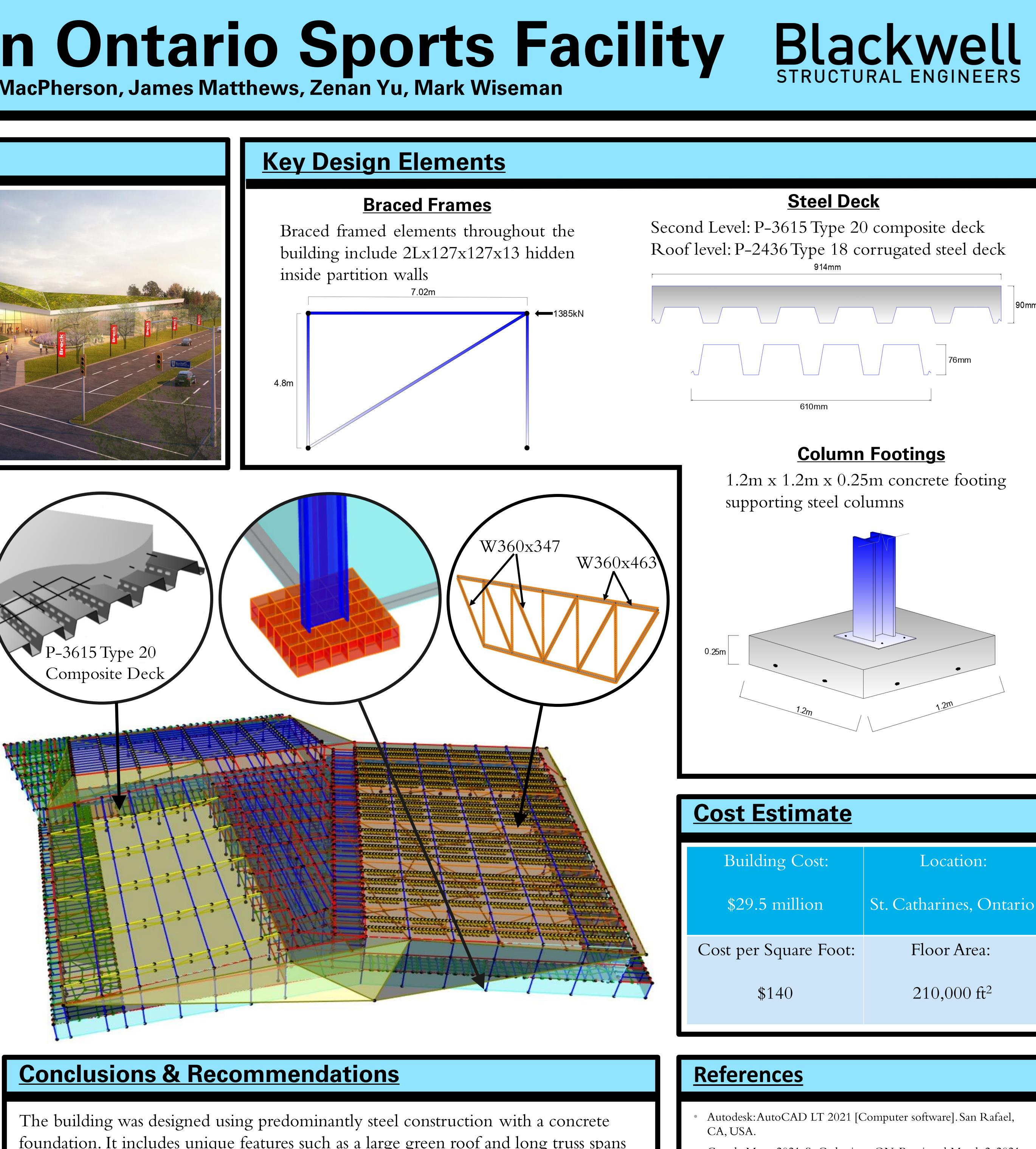
foundation. It includes unique features such as a large green roof and long truss spans over the arenas and gym. The trusses, which span a maximum distance of 51m, are designed to withstand the load from the green roof and are supported by columns that load into concrete footings. The total cost using a type D cost estimate based on the dimensions of the building is approximately \$29,500,000.
