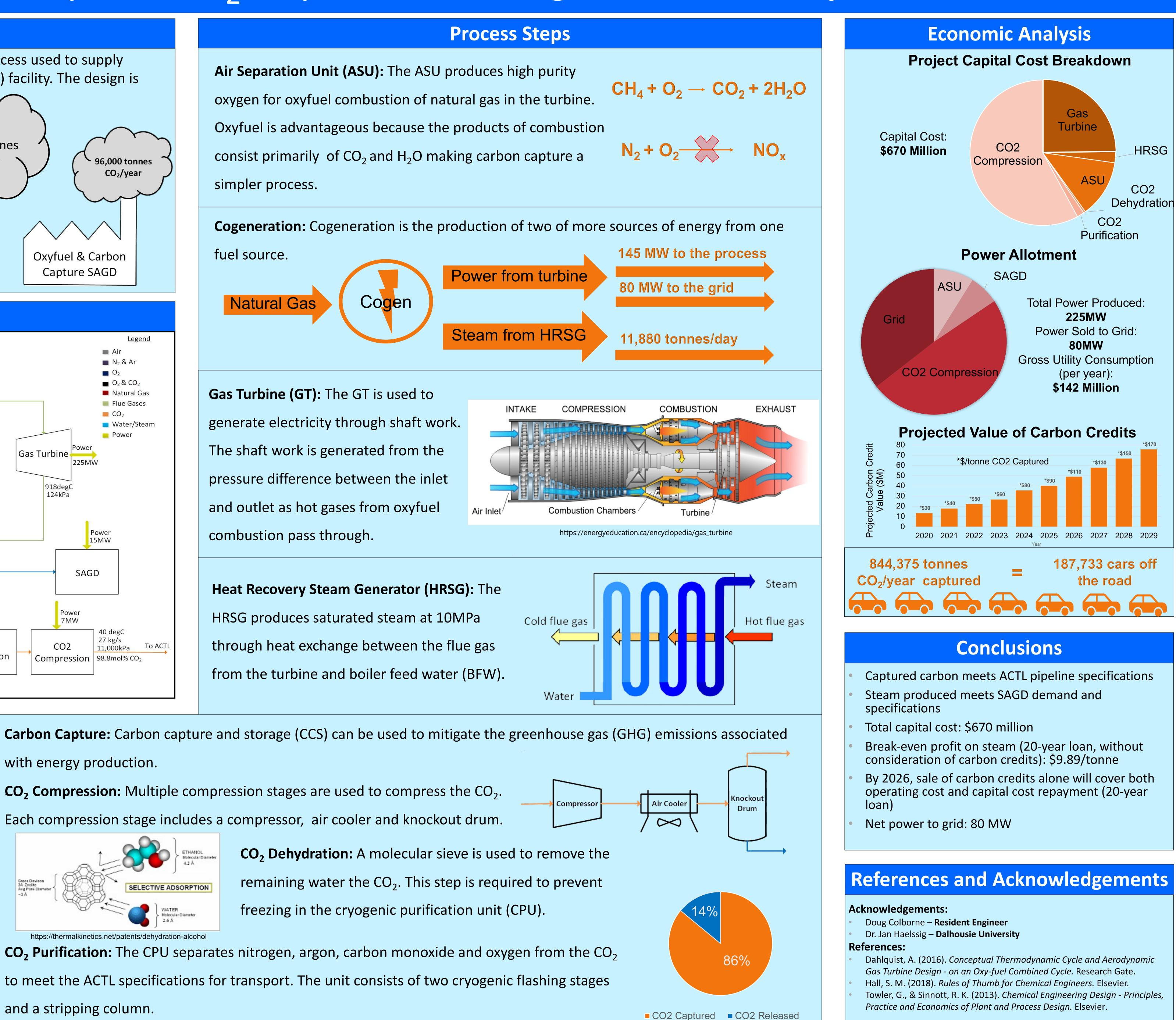
**Gas Turbine (GT):** The GT is used to The shaft work is generated from the pressure difference between the inlet and outlet as hot gases from oxyfuel combustion pass through.
