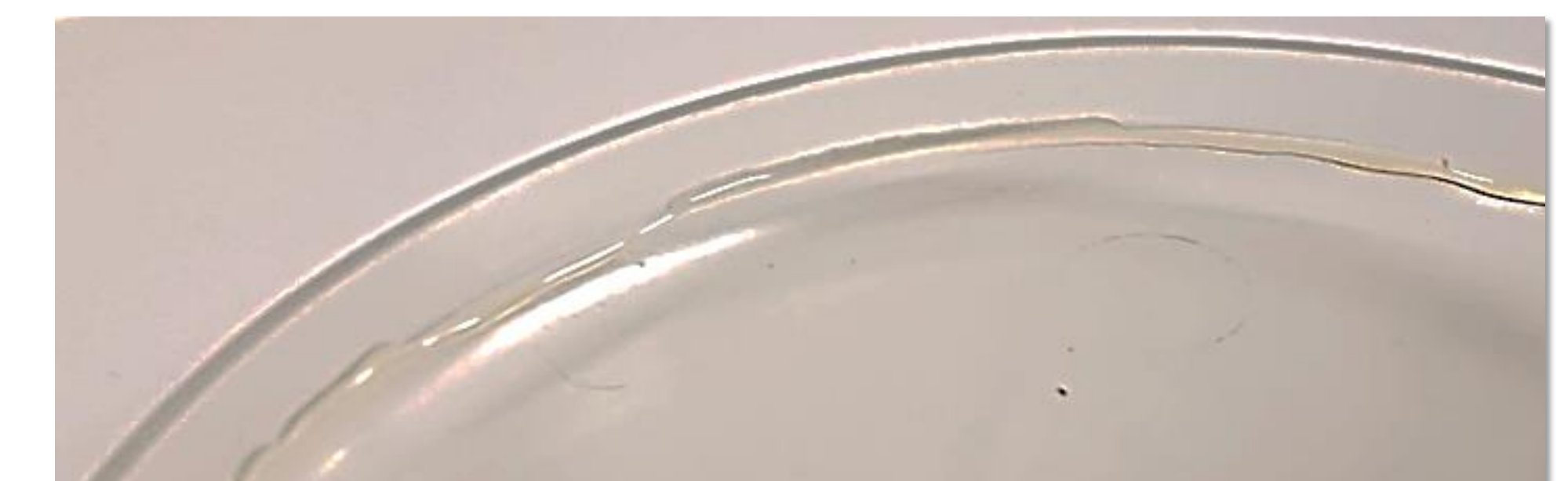
Figure 10 - Corn Syrup Applied to Section of Part
