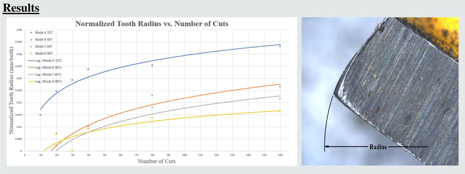
Stereo microscope images were taken of specific teeth on all blades after each cutting interval. The images were imported into SolidWorks and sketching tools were used to determine tooth radius. The graph above shows that low tooth pitch (teeth per inch) blades wear faster than high tooth pitch blades.
