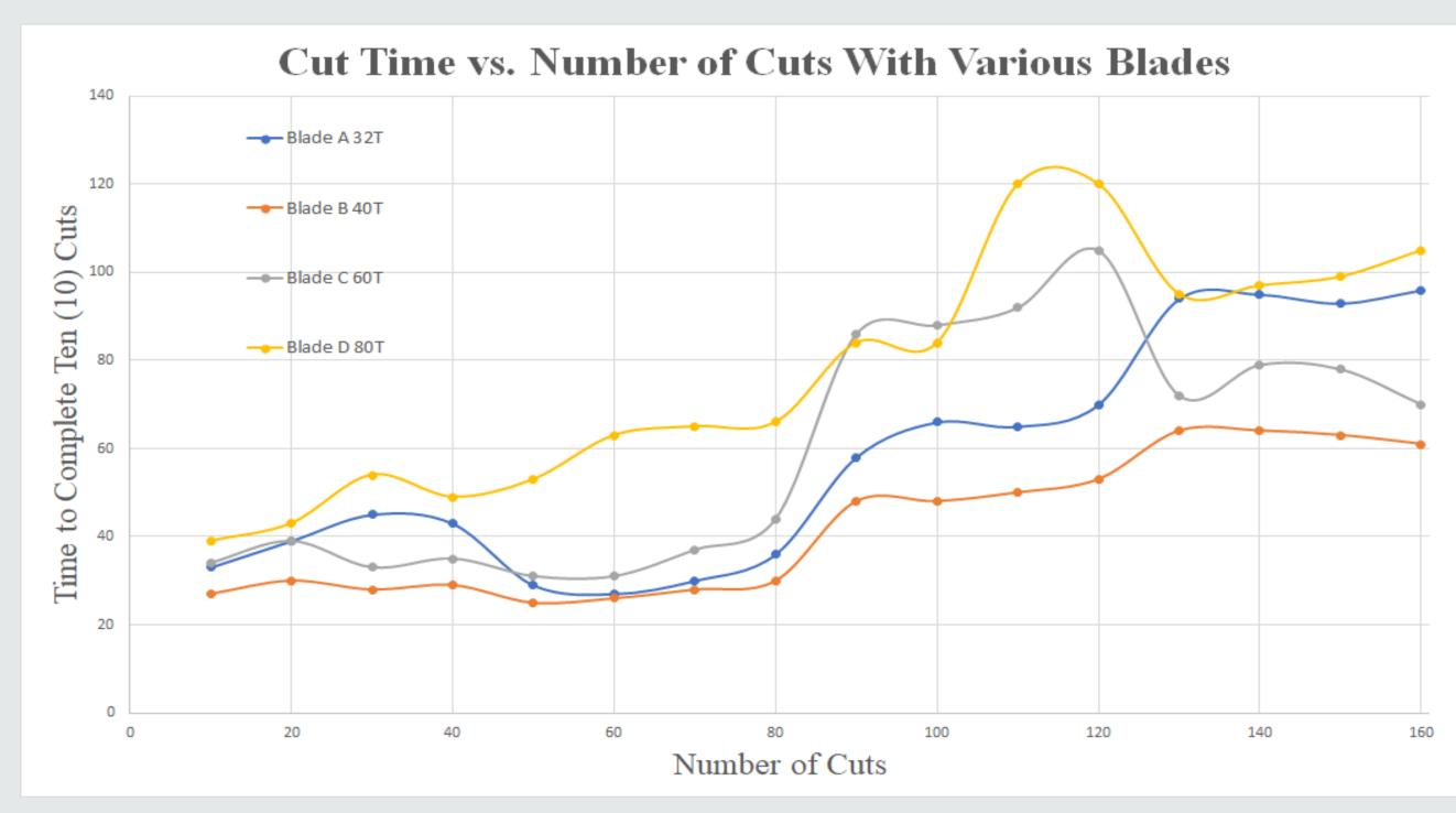
Cutting time increased with the number of cuts preformed on a blade. Blade B cut plastic the fastest, however it's geometry resulted in a rough surface finish. Blade A provided a very fine surface finish, while also operating quickly within its effective lifespan. Blade D gave an excellent surface finish, however its long cutting times precluded it from being a top choice.
