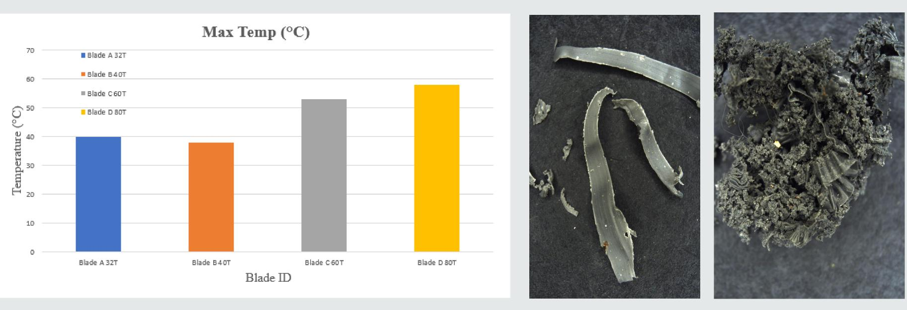
Less teeth tended to produce long continuous chips, which removed heat more effectively. Higher tooth blades tended to melt the plastic, resulting in a build up of molten plastic, which clogged the blade teeth. Rake angle was found to only slightly affect heat generation during cutting.
