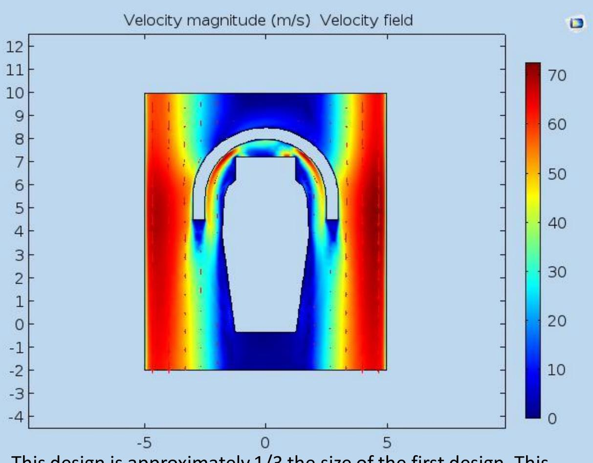
This design is approximately 1/3 the size of the first design. This design takes advantage of the "Coanda Effect". This effect is defined by the entrapment of air as it goes around an airfoil. (Cong, 2019)
